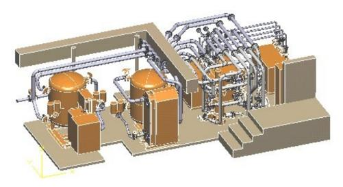
Figure 5 3D CAD drawing of heat pump energy plant design In the last phase of the project the plant was de-assembled, shipped to Cardiff and assembled on site (figure 6).
